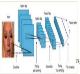
totally seven emotions. The input image will be back and white face image with 48\*48. For each convolution layer we use 3\*3 and for pooling layer we use 2\*2. Both have a stride of 2 . So we initiate the non linearity in the model , use Rectified Linear Unit (ReLU) . R(z) = max(0,z)
