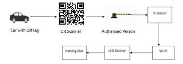
Fig. Structure of Deducting Empty Parking Space
