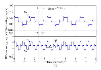
Fig. 2. Experimental waveforms of the dc-link voltage  $v_{dc}$  of the PV inverter operated at 10 % of the rated power (i.e., 0.3 kW) with the MPPT sampling rate of: (a)  $f_{MPPT} = 2.5$  Hz and (b)  $f_{MPPT} = 5$  Hz.
