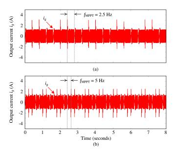
Fig. 3. Experimental waveforms of the output current  $i_g$  of the PV inverter operated at 10 % of the rated power (i.e., 0.3 kW) with the MPPT sampling rate of: (a)  $f_{\text{MPPT}} = 2.5$  Hz and (b)  $f_{\text{MPPT}} = 5$  Hz.
