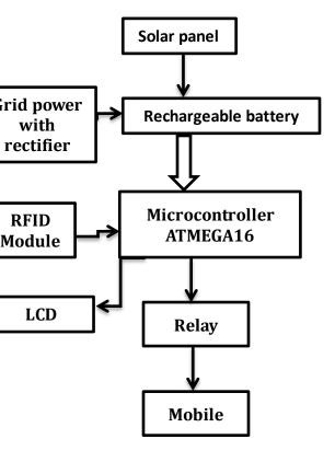
Above block diagram shows the RFID Based Battery charger using Solar Panel and Power supply.
