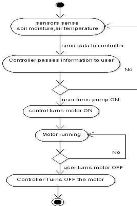
Figure 2: Workflow diagram
