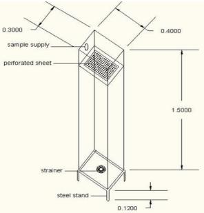
Fig-1: Schematic view of experimental setup
