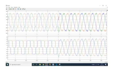
Fig. Source voltages and currents with SRF theory control
