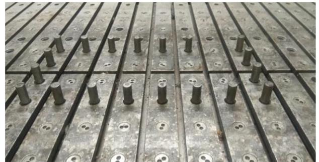
**Fig.4:** Cushion Pins in Bolster
