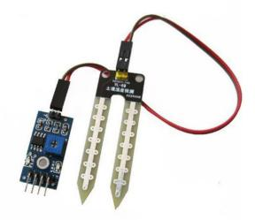
Fig- 2 Soil moisture sensor
