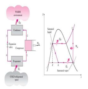
a low- quality saturated mixture. In evaporator, the refrigerant absorbs heat from conditioned space and completely evaporates. Leaving the evaporator, the refrigerant vapor re- enters the compressor at state 1 and finish the cycle.
