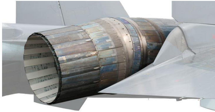
Thrust vectoring nozzle on a military jet.
