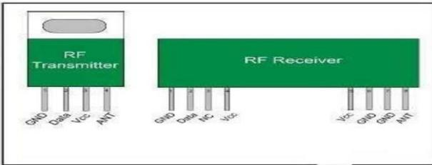
Fig 3.1 RF Transmitter and Receiver
