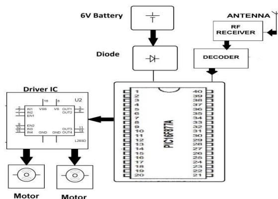
**Figure2. Circuit Diagram of Receiver**
