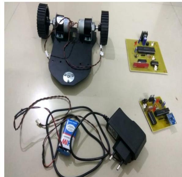
**Figure9.** Unassembled image of robotic vehicle
