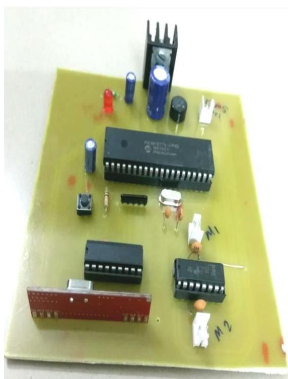
**Figure5. Circuit image of Receiver**
