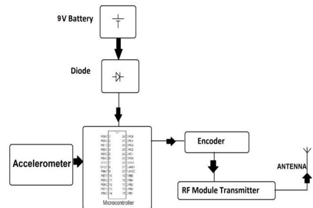
**Figure1. Circuit Diagram of Transmitter**
