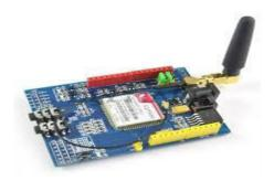
Fig 3: GSM Module
