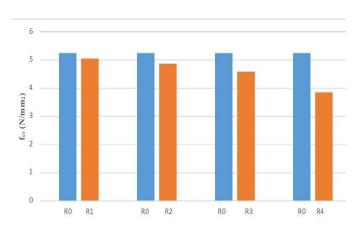
Fig. 4.2.6 fcr of RMSCC compared with SCC after 28 days of curing
