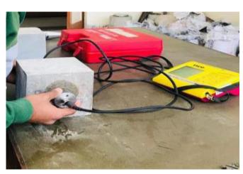
Fig. 4.2.12Performing ultrasonic pulse velocity test
