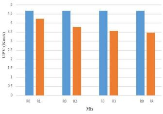
Fig. 4.2.13 UPV of RMSCC compared with SCC
