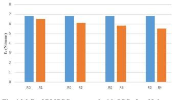
Fig. 4.2.9 fb of RMSCC compared with SCC after 28 days of curing
