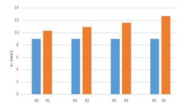
Fig. 4.1.6 tv time of RMSCC compared with SCC
