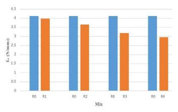
Fig. 4.2.5 fcr of RMSCC compared with SCC after 7 days of curing
