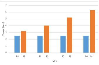
Fig.4.1.3 T50cm time of RMSCC compared with SCC
