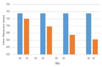
Fig.4.1.2 Flow diameter of RMSCC compared with SCC
