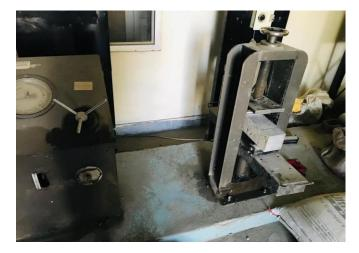
Fig. 4.2.7Flexural tensile strength apparatus
