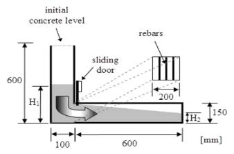
Fig. 4.1.4 Schematic diagram of L-Box apparatus
