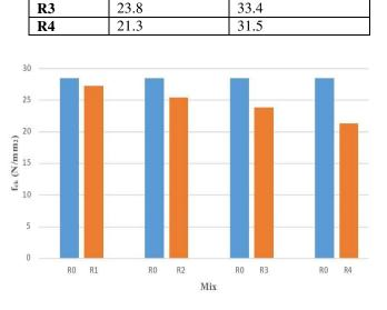
Fig. 4.2.2 fck of RMSCC compared with SCC after 7 days of curing
