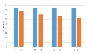
Fig. 4.2.3 fck of RMSCC compared with SCC after 28 days of curing
