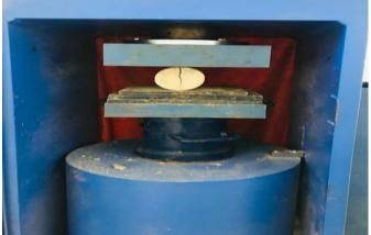
Fig. 4.2.4UTM for split tensile strength test
