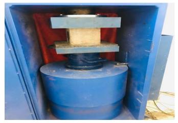
Fig. 4.2.1UTM for compressive strength test
