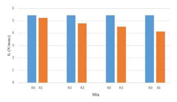
Fig. 4.2.8 fb of RMSCC compared with SCC after 7 days of curing
