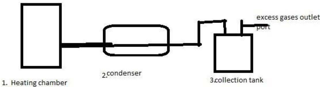
Fig3 line diagram of experimental setup
