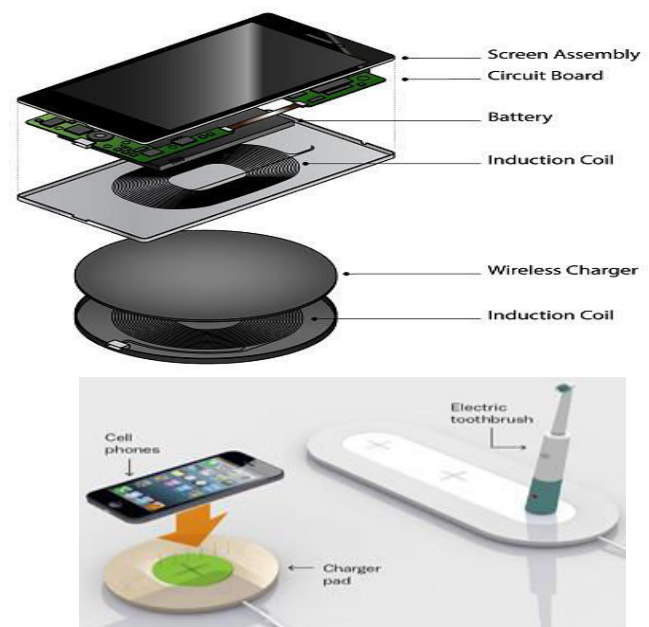
Figure 3: Wireless Charging of transferable device using inductive coupling.
