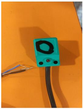
Figure 4: Metal Detector sensor
