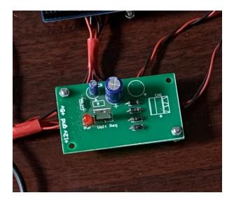
Figure 6: Power supply board
