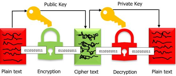
Fig 6: Encryption and Decryption processes in RSA [13]
