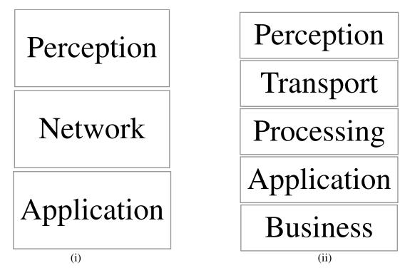
Fig 3: (i) Three-layered architecture; (ii) Five-layered architecture
