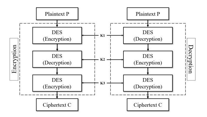
Fig 7: Process of Encryption and Decryption in Triple DES
