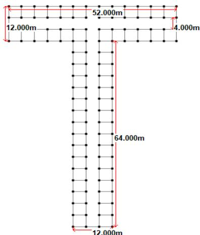
**Fig.1.3 T-Shape Plan**
