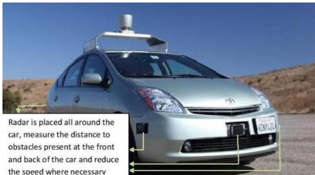
Fig 5: Place of radar sensor
