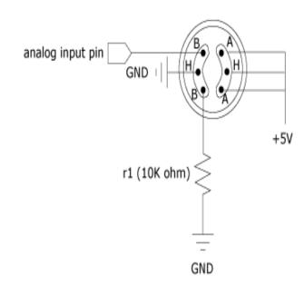
Fig -2: Connection diagram
