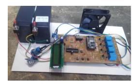
Fig-2: Proposed system of Sewage Monitoring
