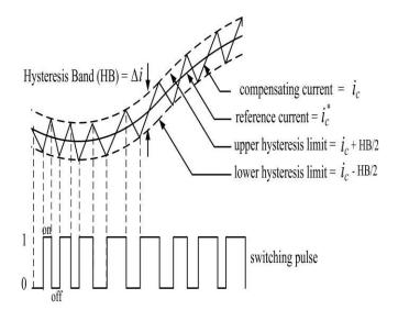
Fig. 3 Principle of hysteresis current control technique
