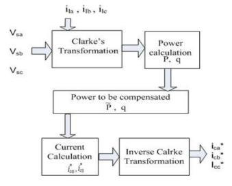
Fig. 5 Basic block diagram of p-q theory
