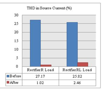
Fig. 16 Comparison of THD in source current
