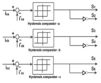
Fig. 4 Pulse generation using hysteresis current control technique
