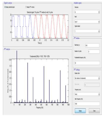
Fig. 9 FFT analysis of source current
