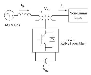
Fig. 2 Basic scheme of series active power filter
