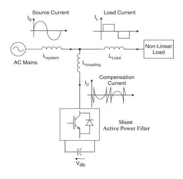
Fig. 1 Basic scheme of shunt active power filter
