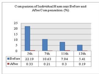
Fig. 10 Comparison of individual harmonics for Rectifier R load
