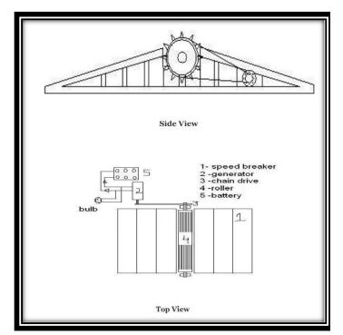
Basic drawing of the structure of prototype working model which includes components such as DC generator, Speed breaker, Roller, Battery, Chain Drive and a Generator.
