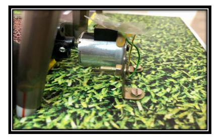
A DC generator is the type of electrical generator that converts mechanical energy into direct current electricity. Here, energy conversion is based on the principle of dynamically induced EMF production.
