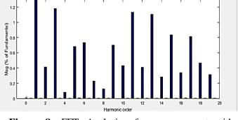
**Figure 8:** FFT Analysis of source current with Detuned filter
