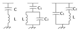
**Figure 1:** Different Filter Topologies (a) ST Filter (b) C Type Filter (c) CCL Filter [5]
