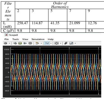
Figure 3: Voltage Harmonics for Phase and Neutral
