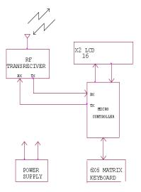
Fig.(b):-Diagram For Slave Station With OUT PC
