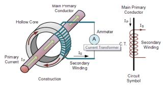
Fig -3: Current Transformer
