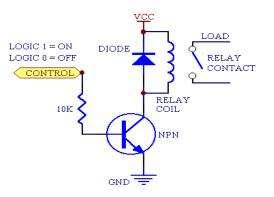
Fig -4: Relay Driver Circuit
