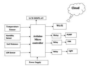
Fig. 4. system architecture
