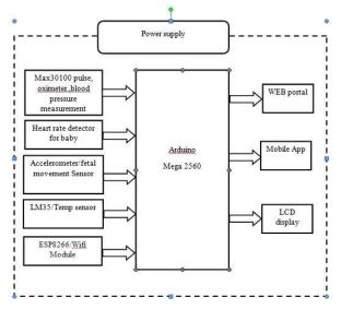
Fig.1 block diagram.
