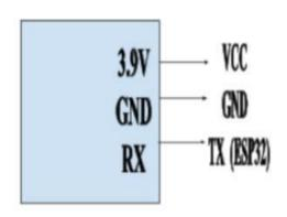
Fig 6. Connectivity block of GSM
