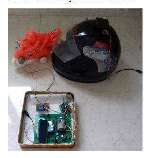
Fig 5.a Helmet with Transmitter and Receiver
