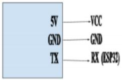
Fig 5. Connectivity block of GPS
