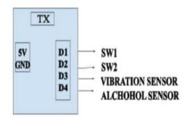
Fig 3. Connectivity block of RF transmitter
