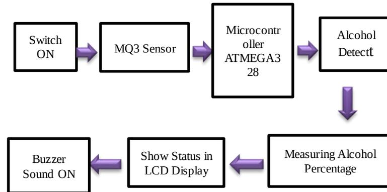
Fig:- Block Diagram Of Smart Helmet.
