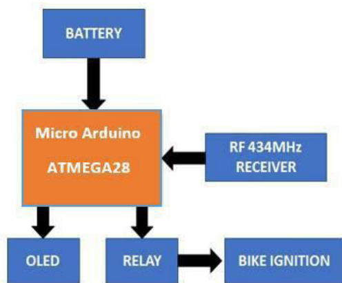
Fig. 2: Block diagram of bike unit
