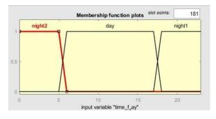
Figure-3: Membership function for the input variable Time
