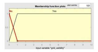
Figure-5: Membership function for input variable Grid Availability
