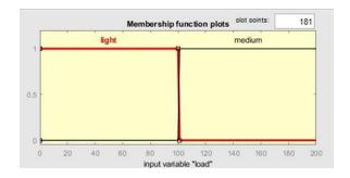
Figure-4: Membership function for input variable Load
