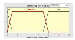
Figure-6: Membership function for input variable Battery Status
