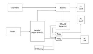
Figure-2: Block Diagram of Proposed SHEMS Framework
