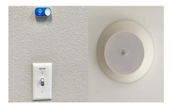
Fig. 4. Some Smart Meeting Room Management System modules. (a) AWS IoT button; (b) Wi-Fi module deployed in the ceiling of a room.
