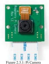
Pi cam is the plug-and-play-compatible device, making it perfect for time-lapse photography, recording video, motion detection and security applications. Connect the included ribbon cable to the CSI (Camera Serial Interface) port on your Raspberry Pi, and you are good to go!
