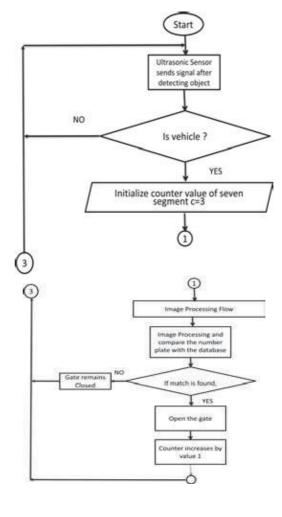
Vehicle Exit Process Figure 2.8.2: Vehicle exit process:
