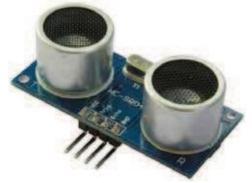
Figure 2.3.3: Ultrasonic Sensor **HC-SR04 Ultrasonic (US) sensor** is a 4 pin module, whose pin names are Vcc, Trigger, Echo and Ground respectively. This sensor is a very popular sensor used in many applications where measuring distance or sensing objects are required. The module has two eyes like projects in the front which forms the Ultrasonic transmitter and Receiver. The sensor works with the simple high school formula that
