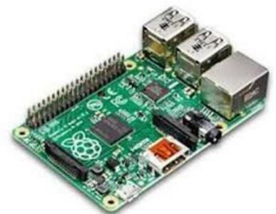
Fig.2. Raspberry Pi Board B.
