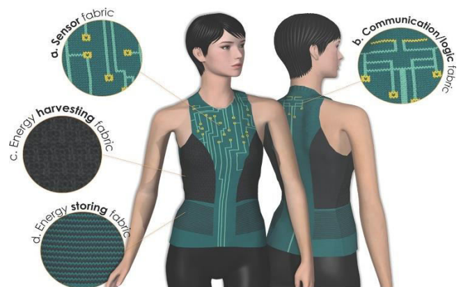
Fig no.8 :- Smart textile with conductive tracks
