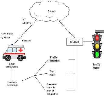
Fig. 1 Working of Traffic Light System
