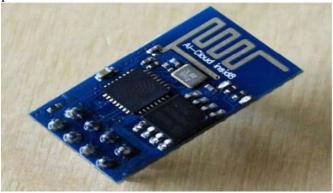
Figure 5: ESP8288 WIFI Modem
