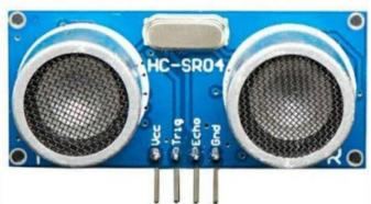
Figure 8: Ultrasonic Sensor
