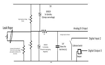
Figure-9: leakage rope circuit diagram
