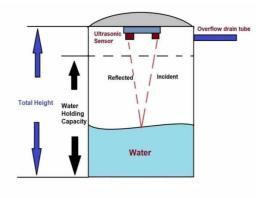
Figure-3: Ultrasonic sensor demonstration
