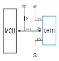
Figure-10: The DHT11 Sensor and outputs serial data
