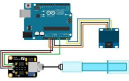
Figure-7: pH sensor circuit diagram
