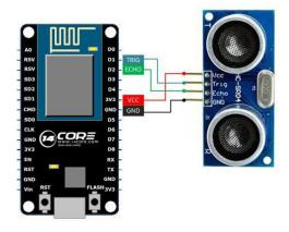
Figure-6: An integrated circuit for ultrasonic sensor
