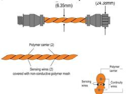
Figure-8: leakage rope construction
