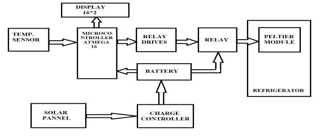
Figure. Block diagram solar based refrigeration system
