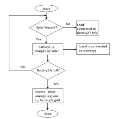
Fig 3: Flowchart of proposed net-metering concept
