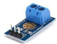
Fig 4 Voltage Sensor
