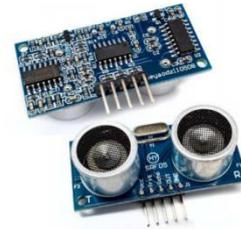
Fig 4-HC-SR 05 ultrasonic sensor
