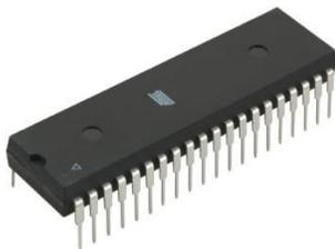
There is a large family of microcontrollers and 8051 is one of those families. The device which we used in our work was the 'AT89S52' which is a typical 8051 microcontroller and it is
