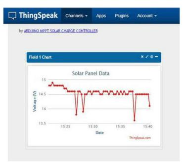
The above fig shows the data chart uploaded to the thingspeak.com voltage vs time. With the help of this we can track the solar voltage remotely from anywhere.
