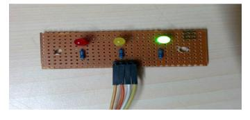
Above fig shows that this project also contains the LED charging level indications of the battery, With the help of led's we can see the battery charging level indication.
