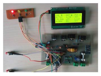
Fig 03. The above fig shows the complete charging system its also provided with reset button in case of program structed we can use of it.
