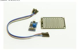
Rain sensor having sensing pad with copper traces mounted on it, together acts as a variable resistor like potentiometer whose resistance varies according to the amount of water on its surface.
