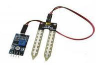
Soil moisture sensors measure the water content in soil, and can be used to estimate the amount of stored water in a profile, or how much irrigation is required to reach a desired amount of saturation. These sensors can be portable and used for instant measurements or installed for long-term monitoring.
