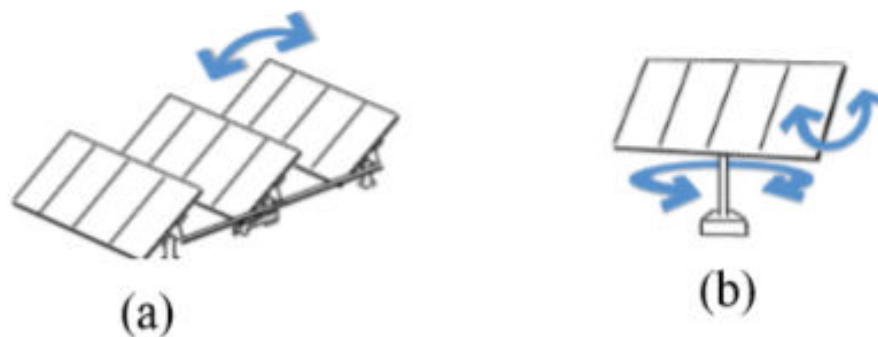
Figure : (a) Schematic diagram of single-axis solar tracker (b) Schematic diagram of double-axis solar tracker
