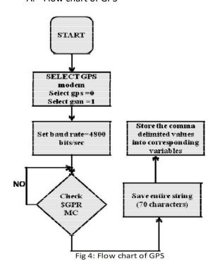
Fig.4 shows flow graph of GPS module which incorporates the calculation of GPS framewrok.[1]
