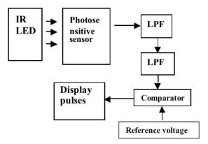
Fig.2: Block diagram of heart beat sensor.
