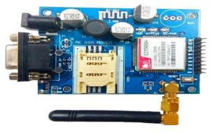
Fig 7: GSM (SIM 900) Module
