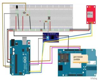
Fig 10: Interfacing LDR, LM35, GSM, And GPS
