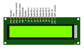
Fig3:Pin Configuration Of LCD
