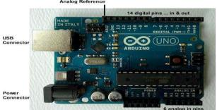
Fig 2: Arduino Development Board
